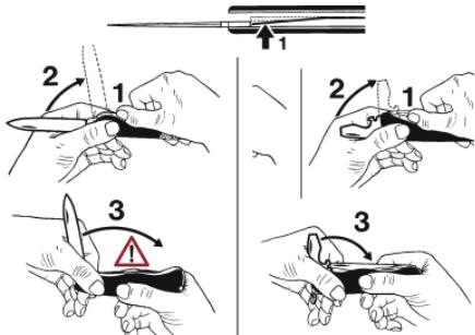
**EN** Stuck blades that do not move easily: open and close a few times in warm water, then dry and oil.
