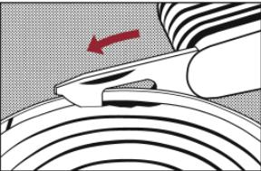
**EN** Place the opener on the can so that the hook gets a firm hold on the underside of the tin; then force the cutting-edge into the lid by gently raising the knife-handle. Important! Keep the cutting-edge close to the rim. Do not cut deeper than the small screwdriver shank.
